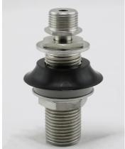
By unscrewing the <u>bottom nut</u> you can remove the <u>inner valve body</u>. Once the inner valve body has been removed it will expose the activation piston.
